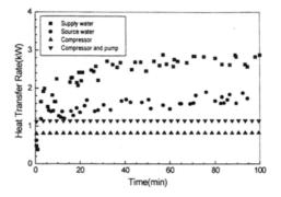
Fig. 7 Variation of heat transfer during the start up of a cycle.
