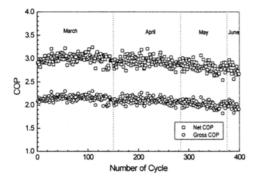
Fig. 9 Variation of the averaged COP during the test period from March to June.
