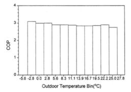
Fig. 6 Averaged COP as a function of outdoor temperature bin during the test period from March to June.
