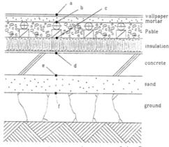
Fig. 2 Cross section view of the floor.
