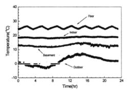
Fig. 10 Variation of floor and indoor temperature during the cyclic operation.
