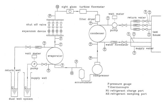
Fig. 3 Schematic diagram of the water-to-water heat pump system.
